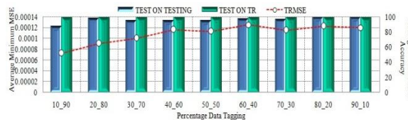
Fig. 12. Variation of average minimum MSE with test on Testing and Training dataset and percent data tagged for training
